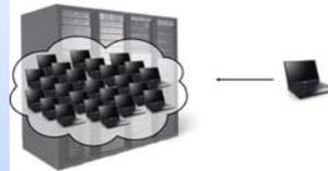
The Early Warning System components are deployed on Virtual Machines. That means they could be easily copied or moved to other Virtual Machine services or Cloud computing services. We have already ported the Virtual Dike, the Breaching simulation and Flood Simulator components to the SARA Clouds.
